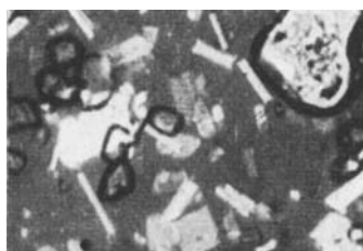
Fig. 2h. \text{CaH}_4(\text{PO}_4)_2 \cdot \text{H}_2\text{O} = \text{Ca}^{\text{I}} (plaques claires). \text{Ca}(\text{NO}_3)_2 \cdot \text{NH}_4\text{NO}_3 \cdot 3\text{H}_2\text{O} = \text{D}^{1-1-3} (rectangles striés). \text{Ca}(\text{NO}_3)_2 \cdot \text{NH}_4\text{NO}_3 = \text{D}^{1-1-0} (cristaux isométriques). \text{NH}_4\text{NO}_3 = \text{NH}_4^{\circ} (gros blocs).
